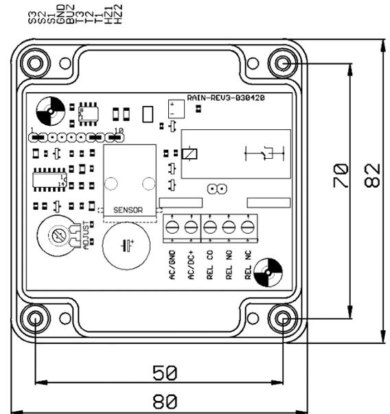
**Sensitivity setting:** The sensitivity of the humidity signal can be influenced at the potentiometer. A higher sensitivity is achieved by turning the potentiometer axis counterclockwise (right = high sensitivity, left = low sensitivity). The middle position is most suitable for normal rain signaling. Note that there is no function at the end stops!
