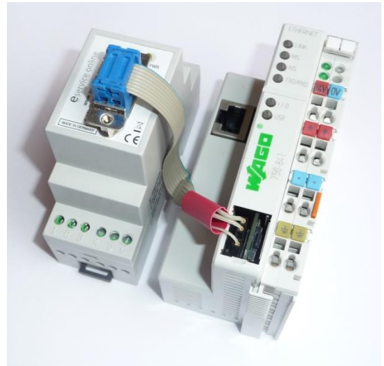
Bild: Systemmontage 1-Wire Buskoppler – SPS
